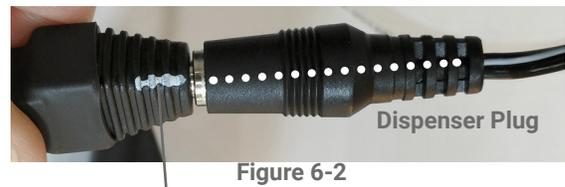
Battery Power Supply Plug - Align white mark with white wire on dispenser plug
